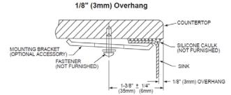
NOTE: THIS UNDERMOUNT SINK IS DESIGNED TO MOUNT TO SOLID SURFACE (NON-LAMINATE) COUNTERTOP ONLY.
